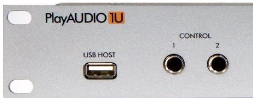
Use the PlayAUDIO1U CONTROL ports with compatible footswitch(es) to send CC/PC messages, arm or disarm automatic failover, load CC / PC, or Toggle scenes
