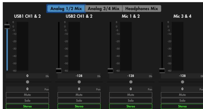
Select Analog 1/2 Mix to show a list of configurable output channel signal sources and edit the level, pan (if **[Stereo]** is selected), **[Mute]**, **[Solo]**, and **[Stereo]** selection for outputs 1 & 2 as indicated below.
