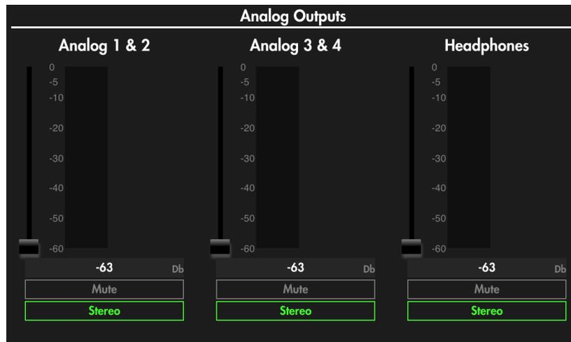
Pictured above are the LED meters and respective faders to control output level per output. Output level can be adjusted by dragging the on-screen fader up or down, or by clicking the current Db value in the gray box directly below the fader and volume meter output array and typing in the Db amount you want for gain in the range -60 to 0 Db.
