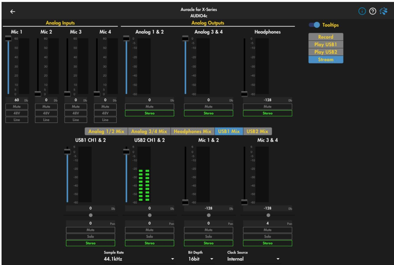
Stream mode output with USB1 mix visible with [Stereo] selected. USB2 mix options are identical to USB1 mix options in Stream mode. A computer is plugged into USB2. USB2 channels 1 & 2 are seen metering in the bottom row.
