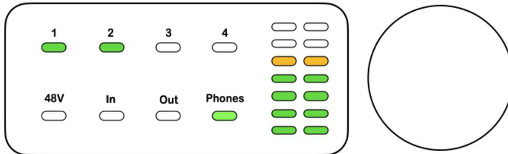
**Signal Level Mode:** Touch the region centered around [**Phones**] on the bottom row of the Interactive Display until the [**Phones**] indicator turns green. A green [**Phones**] LED indicates that the LED meters are in **Signal Level Mode**. In this mode the LED meters will display the level of audio being sent to the [**Phones**] socket on the rear of the AUDIO4c.
